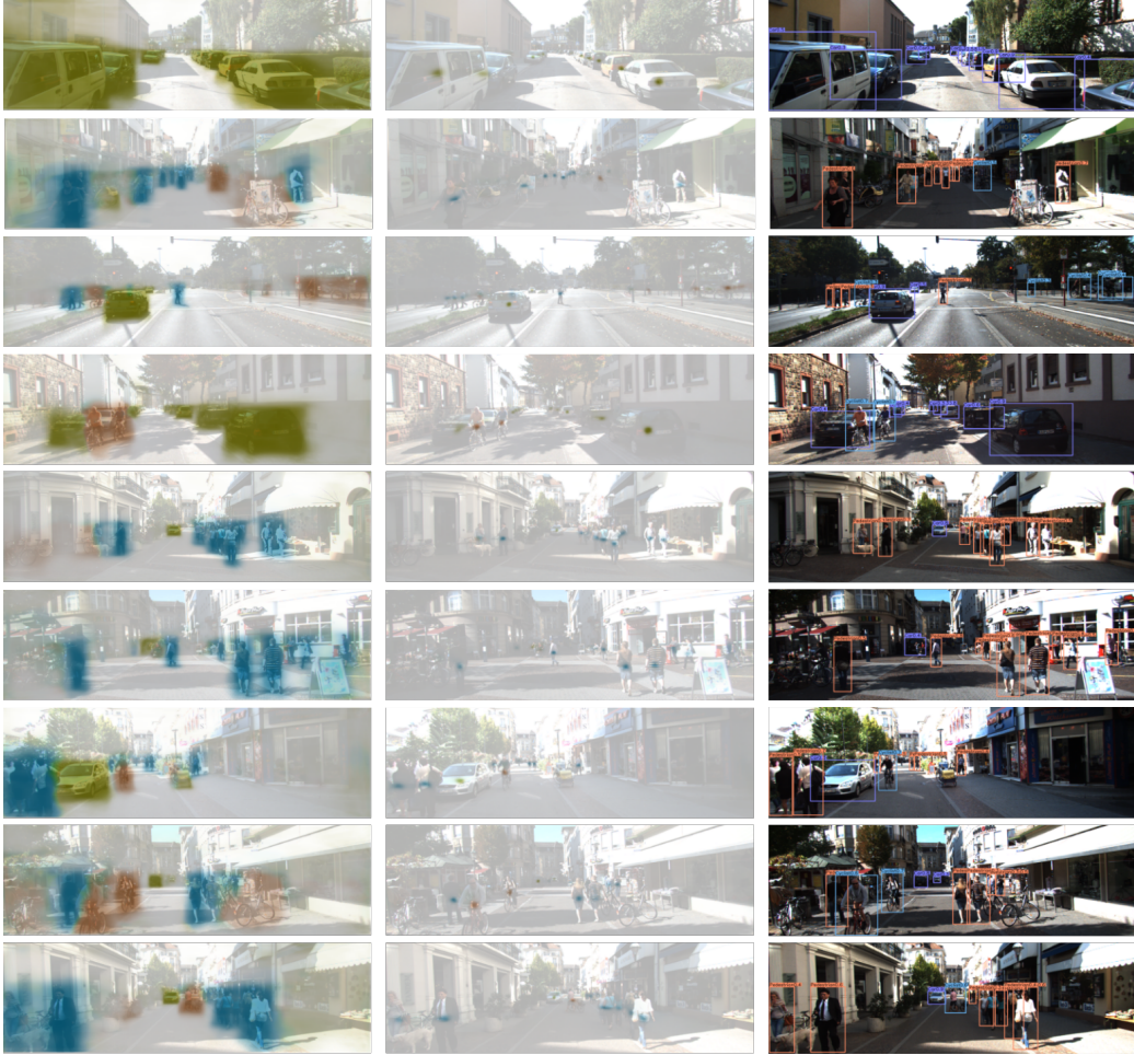
Fig. 6. Visualization examples of FII-CenterNet for traffic object detection. Left: the result of foreground region proposal; Middle: the detected center points; Right: the final detection result.
